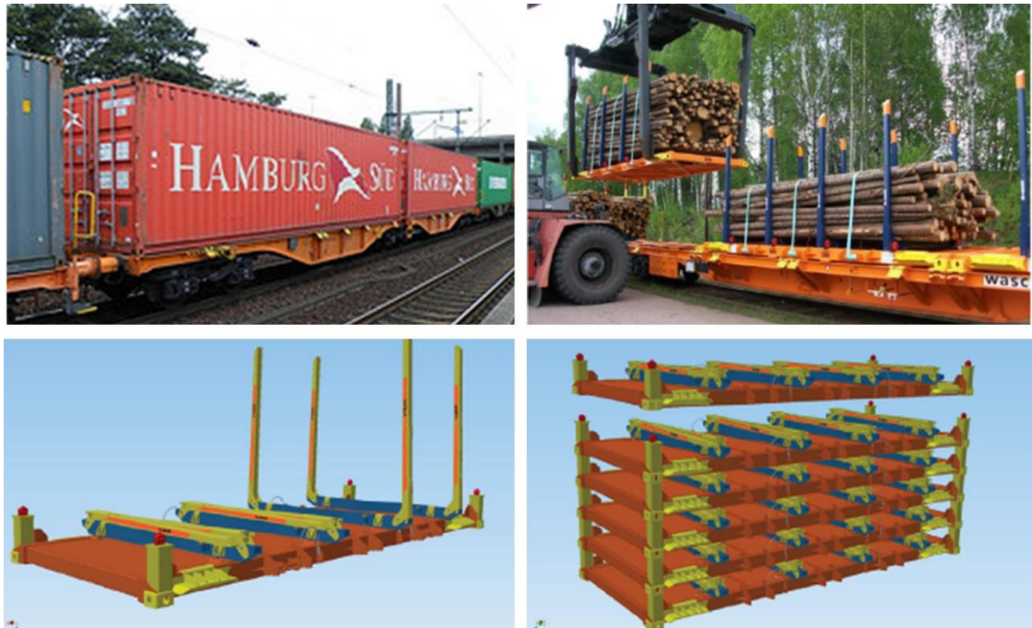
Fig. 1. Foldable stanchions Wascosa stackable flexi freight system ® . Source: Wascosa.
