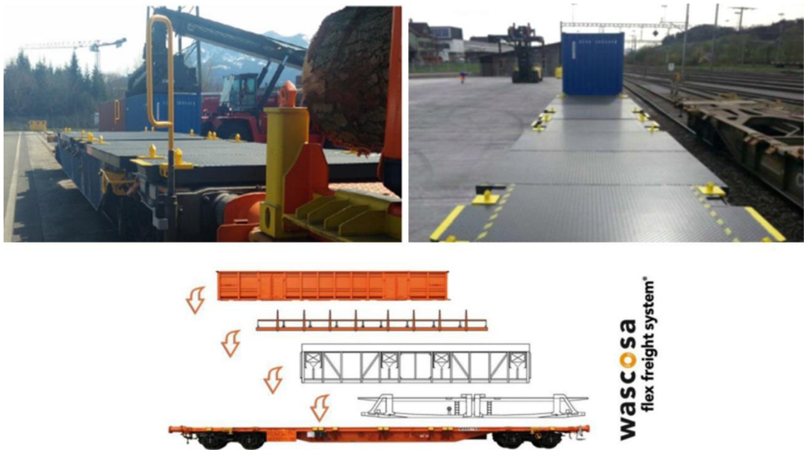
Fig. 2. Container loading adapter to flex car. Source: Wascosa.
