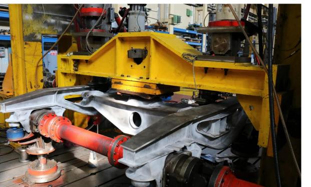
**Bogie frame fatigue testing at VUZ**
